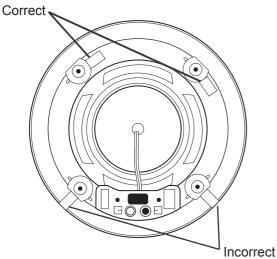
With the grill removed, place the speaker in the ceiling opening. Make sure that the speaker wire is not hanging against the speaker where it can vibrate and rattle as the speaker reproduces your audio program.
